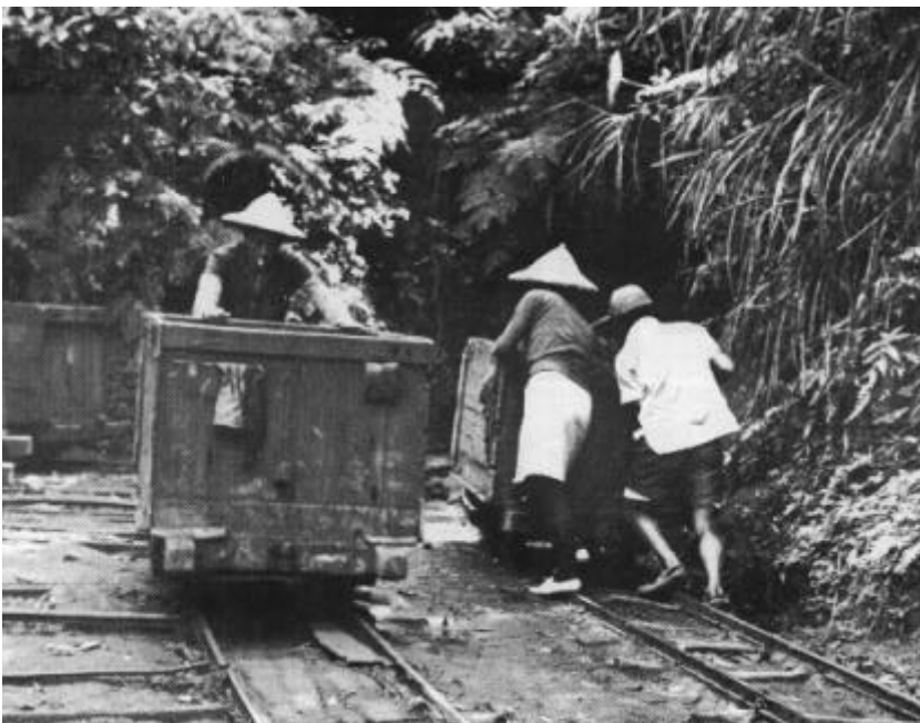
fig. 6 – The helper (female) and the regular locomotives have been waiting for a northbound empty to clear the tunnel. Now that it has emerged they have a hard job starting the train for its tunnel transit. The helper only goes as far as the tunnel portal.
