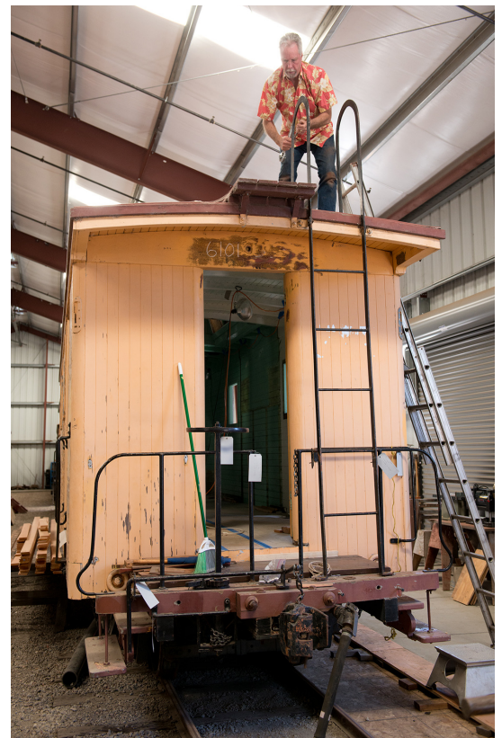
Jack Burgess begins to remove a ladder from the body of caboose 6101. Select pieces of car hardware will be either modified or completely rebuilt to conform to new target restoration dates, ca 1910-1913.
