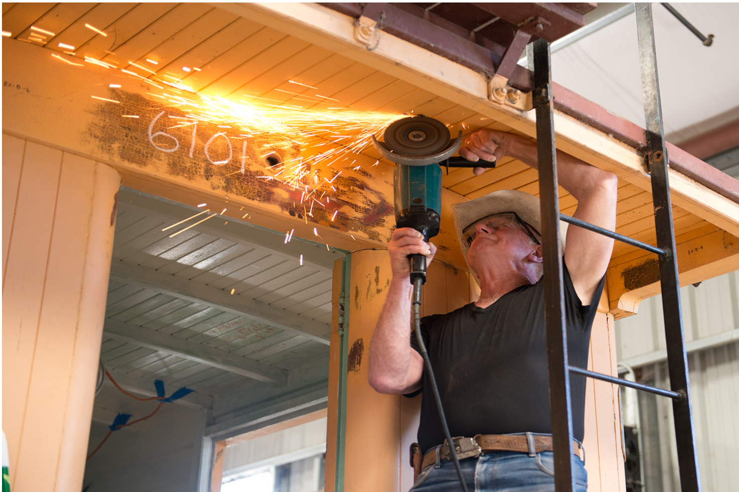
Bruce Sorrel removes bolts holding 6101's end ladder in place
