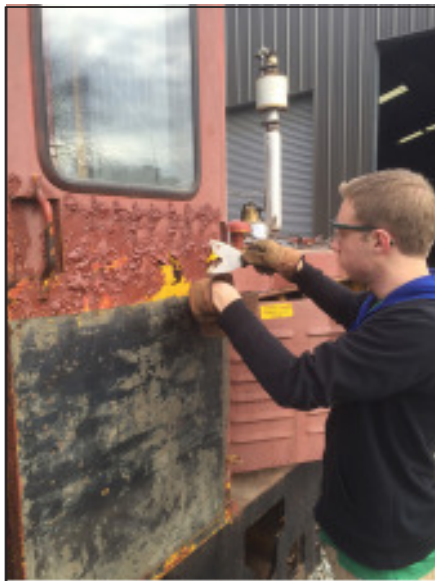
Bobby Goldie scrapes rust away by John Goldie
