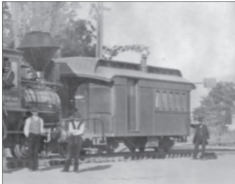
Caboose 1009 as it appeared on the San Joaquin & Sierra Nevada Railroad, circa 1890s. While built with a bullnose roof style, visually different from caboose 47's duckbill roof style, both cars have nearly identical body dimensions, and many similar construction details. Caboose 1009 eventually went to Southern Pacific narrow gauge, and was rebuilt a number of times before retiring from active operation in 1960, at the end of SP ng operation. At the time of its retirement, it carried the road number SP 401.
