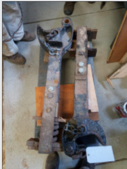
Both couplers removed and ready for storage.
