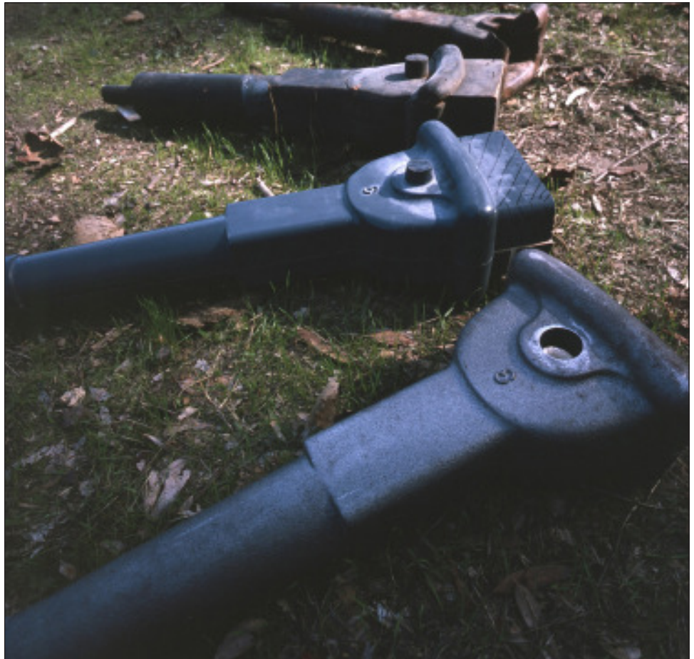
A good example of the parts collection in action is this circa 1985 image of how a replica Carter Brothers coupler was created by our Museum from historic parts. At the far back of the photo is a damaged West Side original Carter link and pin coupler (also called a draw bar), installed as new equipment by Carter on a set of 24-foot-long flat cars delivered to West Side in 1898. Next in line (coming towards the camera) is an original West Side pattern that captured many (not all) features of the original Carter coupler, allowing West Side to reproduce the couplers as they became worn out or broken. Next in line is our modern pattern, created from the first two historic originals. And finally (closest to the camera) is a casting made from our modern pattern. A pair of these replica draw bars now operate on D&C flat car 64. Photo: Bruce MacGregor
