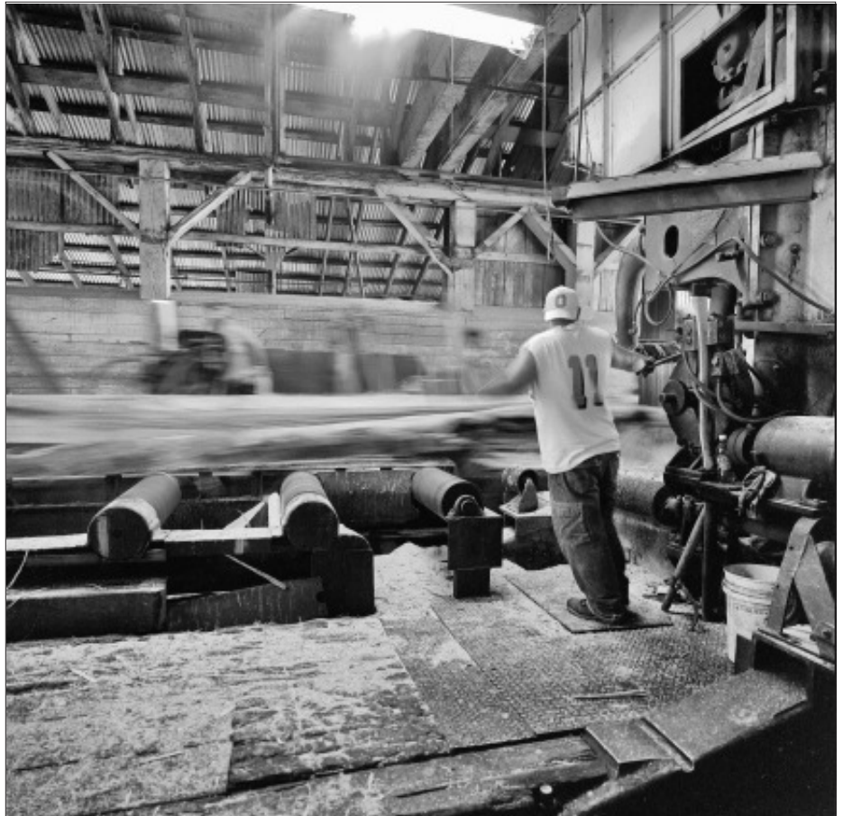
Main saw carriage at the Hull Oaks Mill near Corvallis, Oregon. Photo: Bruce MacGregor
