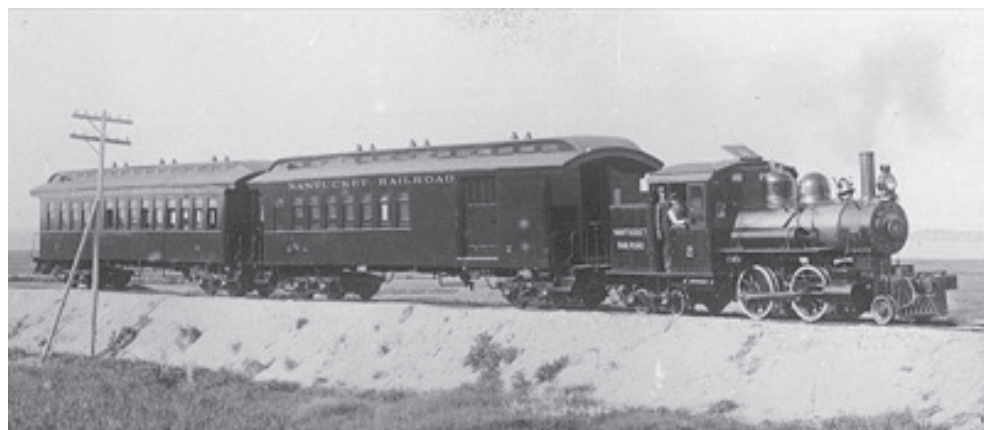
American Locomotive Company 2-4-4, presumably the third No. 2. Credit: Nantucket Historical Association Library
