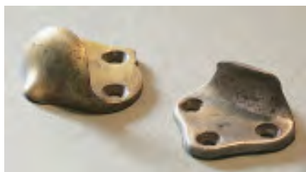
Post & Co. window latches, used on an 1879 Carter coach with duck-bill roof.
