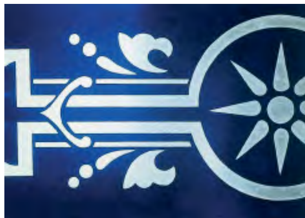
Transparent, etched-glass clerestory window used on an 1879 Carter coach with duck-bill roof.
