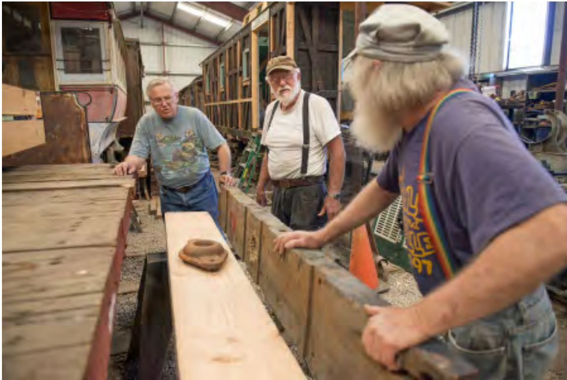
Gene Bobik, Tony Peters, and Gene Arrillaga (left to right) lay out the new bolsters (Gene A has both hands on the old bolster). They are laying out the hole which the center plate for the truck will fit through (the center plate is shown on top of the new bolster). In the background on the right, is caboose 6101. Oakland Railroad 12 horse car (built by J. Hammond car works) is on the left.
