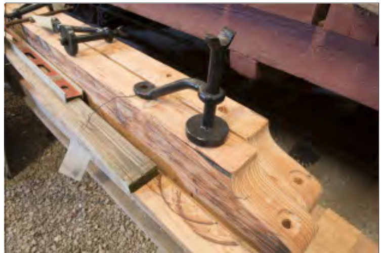
Caboose 6101 new needle beams and queen posts. Photo: Bruce MacGregor
