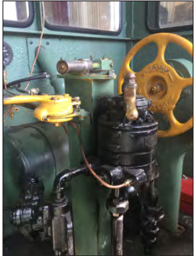
New automatic brake valve in Katie.
