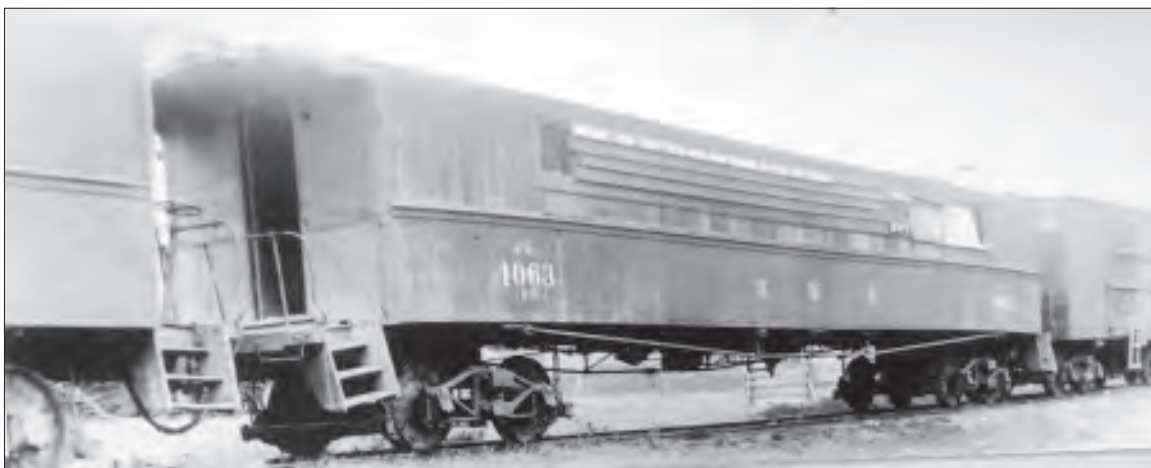
The onetime NPC/NS picnic-excursion car No. 43 (and a like sister car, far left) was photographed somewhere on the standard gauge Northwestern Pacific in lowly maintenance of way or “MW” duty, sometime after 1908 but possibly c. 1925 or later. The placement of standard gauge arch bar trucks underneath have hiked both cars far above their original passenger service height and an overall state of “droop” and neglect clings to the 1063. With its broad observation “windows” sealed up with miscellaneous lumber and shingles, it seems to have been in use as a crew bunk car. Its ultimate fate remains unknown, but being burned for salvage scrap metal before the 1940s seems likeliest. Photo courtesy NWPRRH Archive collection.
