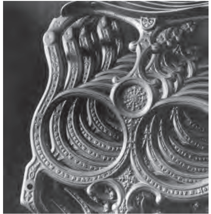
Finished Buntin seat reproductions, cast by Sunset Foundry. Photo: Bruce MacGregor
