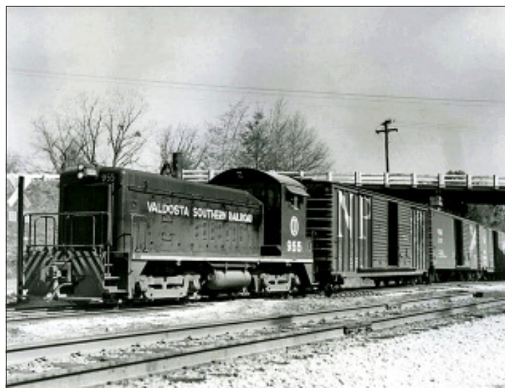
In this circa 1960 view, Valdosta Southern SW900 No. 955 picks up an interchange cut from the Seaboard Air Line at Madison, Florida. The 115 ton diesel ran on 60-pound rail between Clyattville and Madison as needed. Note the O-I logo of parent company, Owens Illinois, Inc. Photo by Dr. William J. Husa, Jr.
