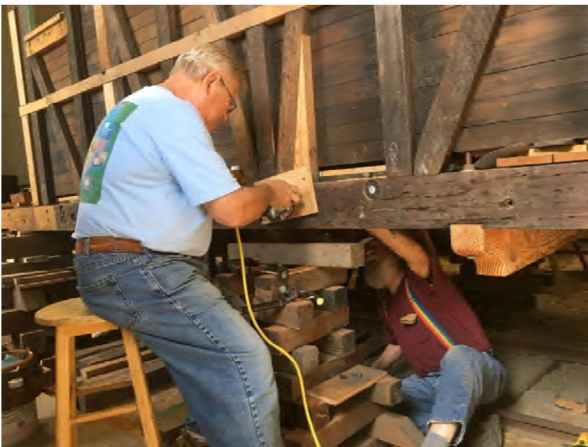
Gene Bobik (left) and Gene Arrillaga (under caboose) work on improving a strengthening attempt made to 6101 earlier in its life. Photo: David Waterman
