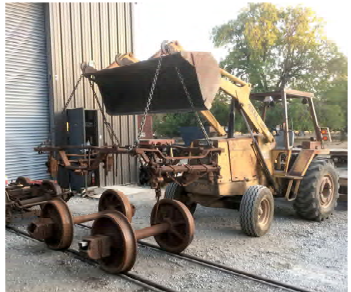
Rotating the wheel sets to use under NWP caboose 6101 currently under restoration. Photo: David Waterman
