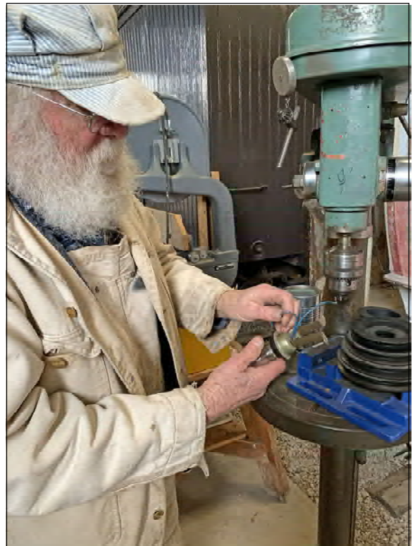
Gene Arrillaga discovered a stripped wire inside the drill press. He is also going to install new belts, but getting the correct size is proving to be a challenge. You can see a couple of belts that were incorrect even though the catalog said they would fit.
