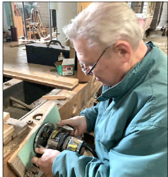
Gene Bobik tests the depth of the router before using it to counter-bore another hole in the side sill.
