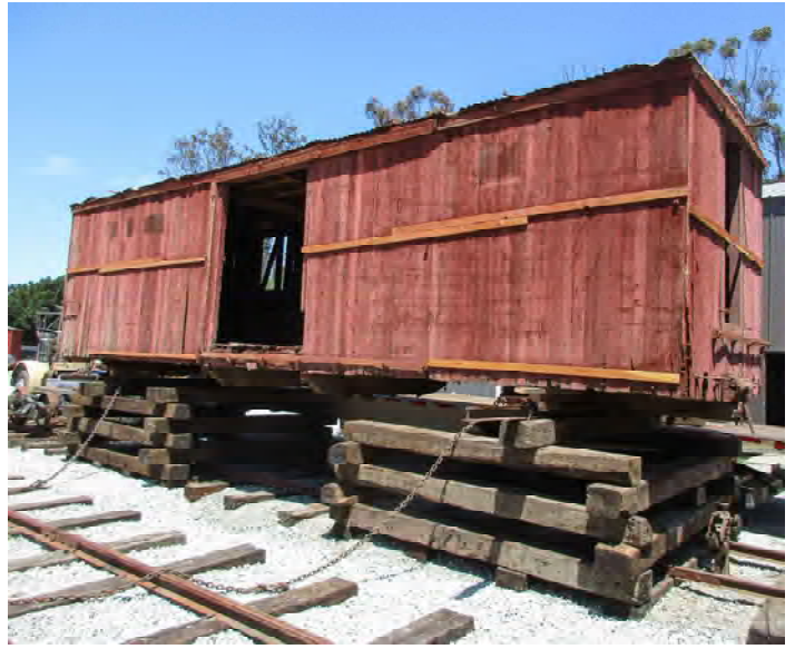
The box car is now on the cribbing. Next step is to jack it up and remove the pieces of rail underneath. Photo: Don Marenzi
