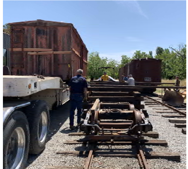
The truck is parallel to the track then car was jacked up enough to slide two 20 ft rails underneath. Photo: Editor
