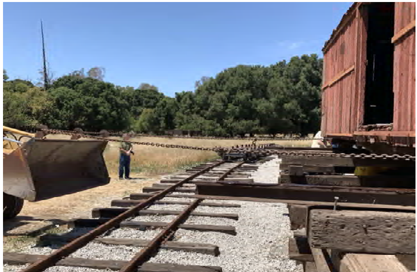
Using the tractor, David is pulling the car from the truck over to the cribbing on top of the rail while Don Marenzi watches. Photo: Editor
