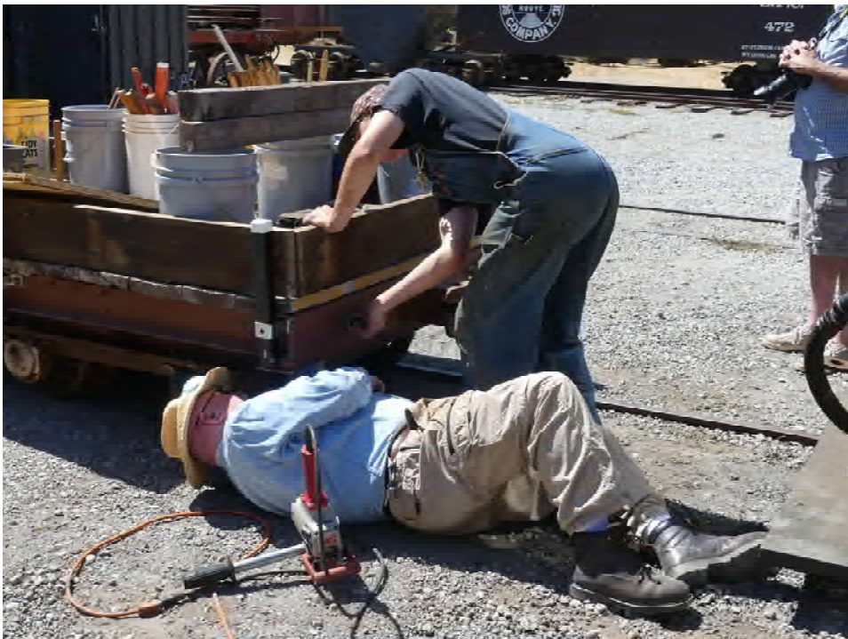
David Waterman (standing) and Ron Quilici install end board brackets on the new tool car. Photo: JS Burgess
