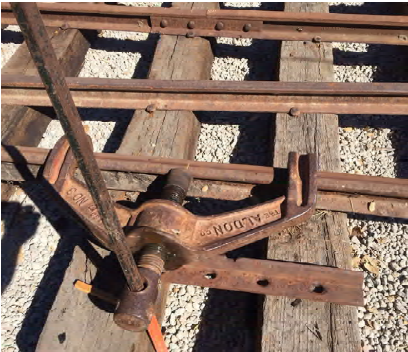
Manual rail bender at work. This style is no longer made--it has been replaced by a hydraulic cylinder (one of the track crew's wish list items). These are used to make curved rails and also to set the kink where the point nests in.
