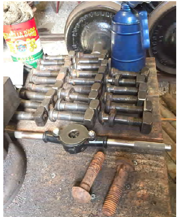
Bruce Sorel has been cleaning up our track bolts. Note the before and after at the bottom of the photo.
