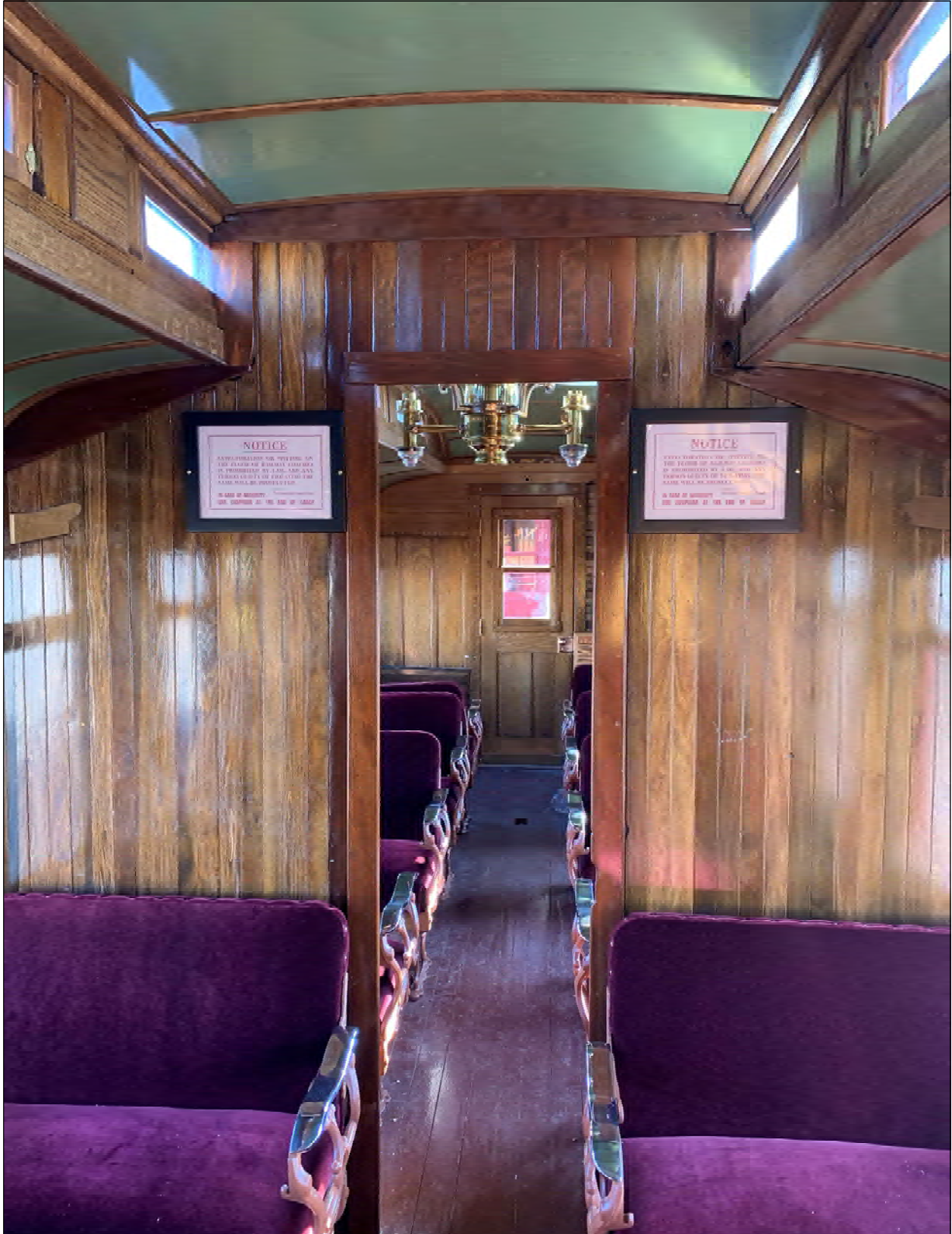
The completed interior of D&RG coach 256 with the Buntin seat castings. Photo: Stathi Pappas, Cumbres & Toltec
