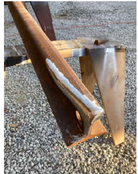
Detailed view of the end notch for a guard rail. This is made by a band saw cut followed by grinding.
