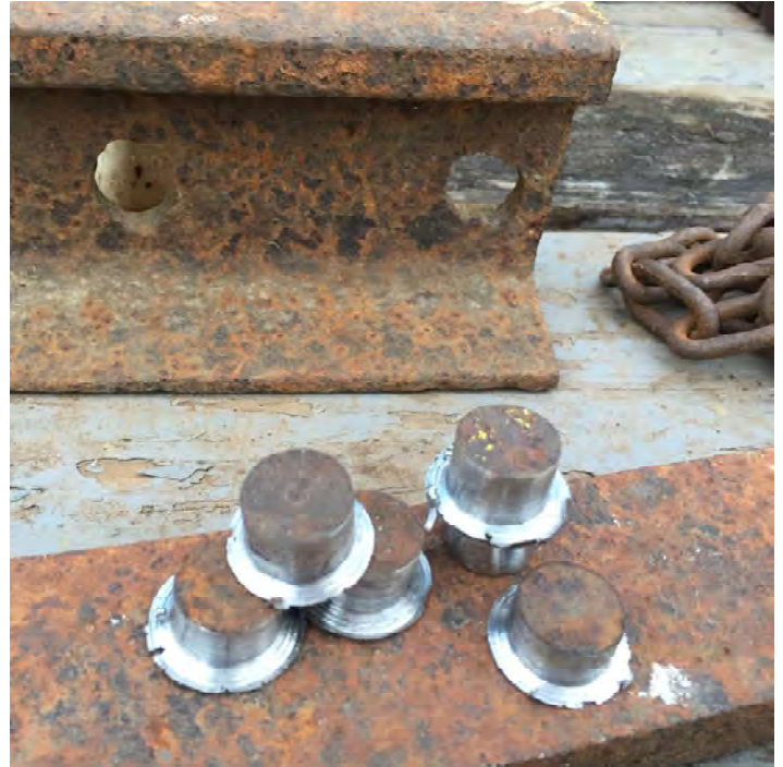
The drill hole slugs. We are still on our first hole cutter bit. It takes 30 seconds per hole!
