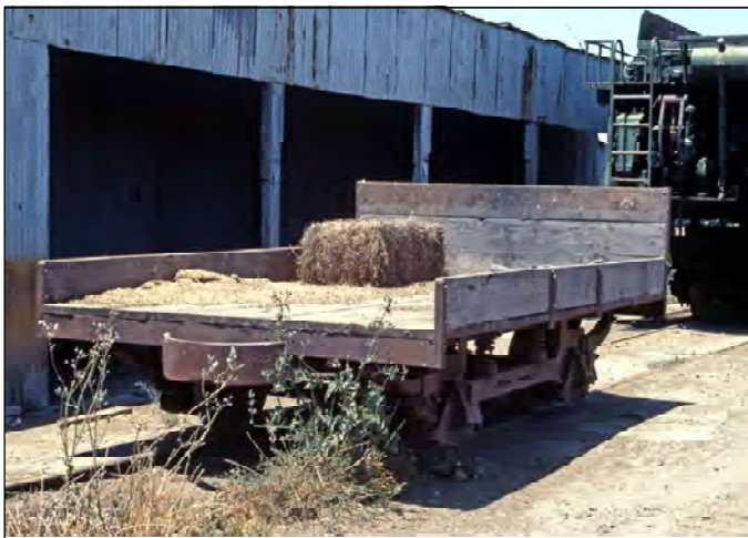
Flat car built on a Los Angeles Railway trolley truck
