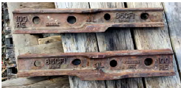
Image 1: Left Side Field (3L) and Gauge (4L)—commercial-built compromise joint bar set.
