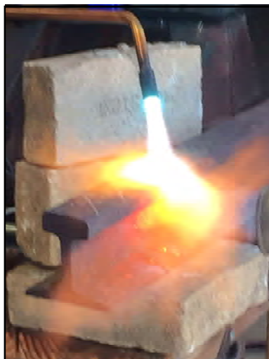
4/11 workday: rail bending heat test - not hot enough. Photo - John Goldie
