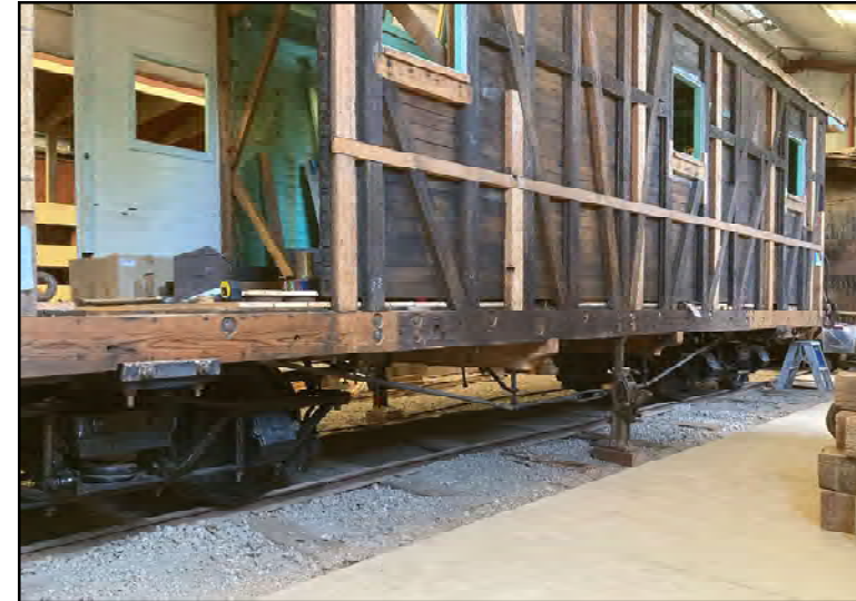
The truss rods for Caboose 6101 have been straightened and re-bent to accommodate the replacement queen posts that were installed to back date the car to its early NPC appearance. The car now has its full framing strength back which will allow work to proceed on other areas of the car. Photo - David Waterman
