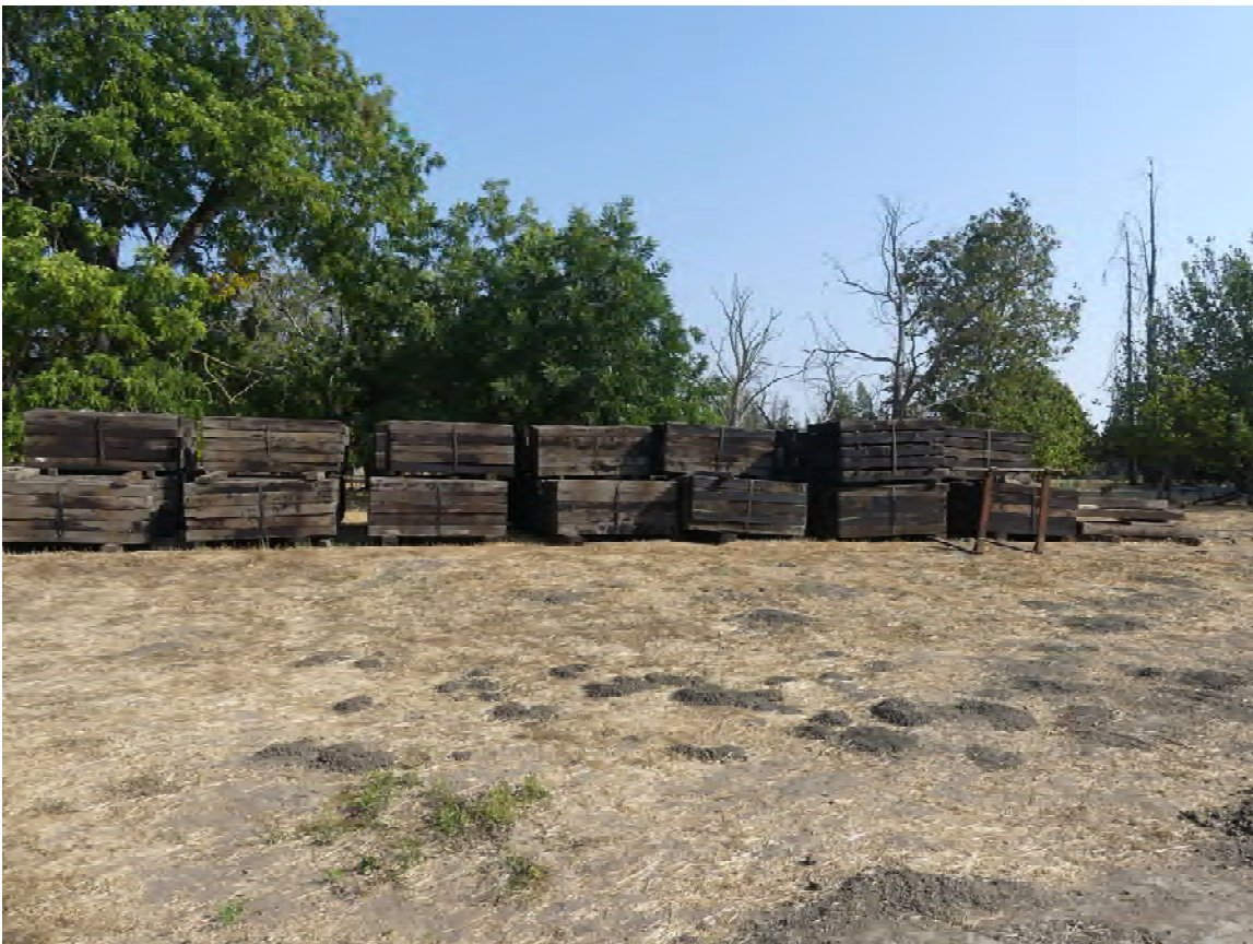
This is our stock of 6-foot relay ties that we acquired last year. The mainline extension from the road west to the spring switch will utilize them. The rest of our railroad has 8-foot standard gauge ties, but the 6-foot ties give our railroad a trim, narrow look. Photo: JS Burgess
