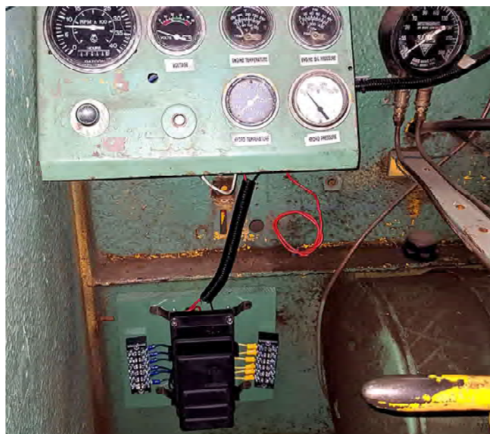
Katie's new relay and fuse box for the headlights, fan, dome light, and wipers.
