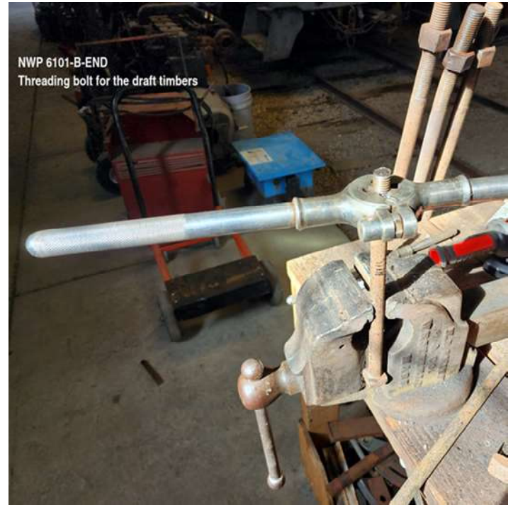
Rethreading bolts for the platform draft sills.Andy got to use the newly donated angle grinder. Photo -AJL Cary
