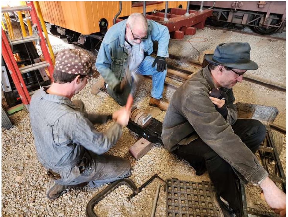
Inserting the coupler spring. David Waterman and Tony Peters pound while Damian Stellabott holds down the coupler (with a broken hand!). Photo - AJL Cary
