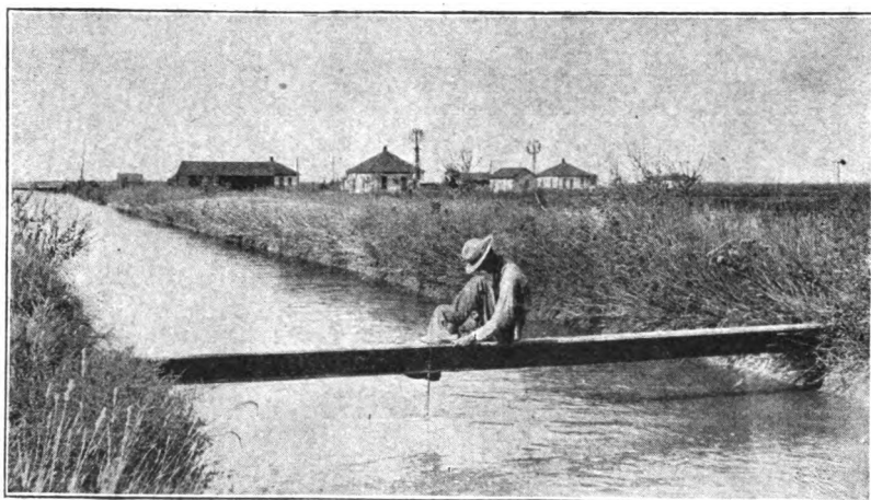
Fig. 42. Measuring Discharge of Irrigation Canal with Current Meter
